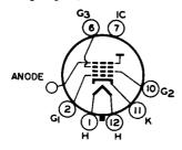
Pin 1: Heater Pin 2: Grid No.1 Pin 6: Grid No.3
